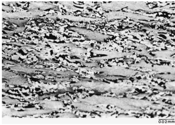
Fig. 2 Microstructure of dual-phase steel after intercritical annealing at 790 °C followed by 48% rolling reduction and quenching in boiling water
